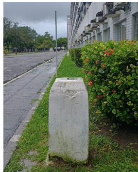
Figure 1. The calibration baseline is composed of seven pillars with forced centering, in June 2024.
