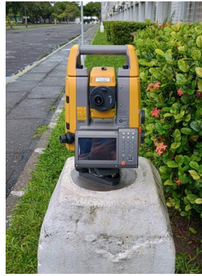
Figure 2. The Topcon GT-605 RTS used in the measurements, in June 2024.
