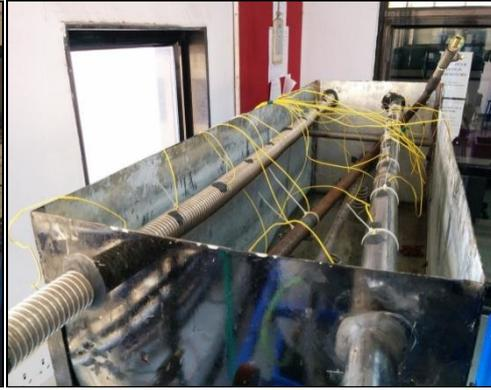
Fig.7 Thermocouples on Pipes
