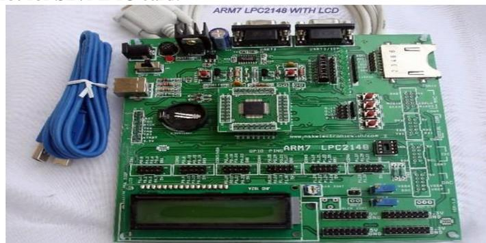
Figure 1. ARM microcontroller
