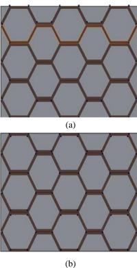
**Figure 2**(a). Spot weld location (dark spots) between core andtop panel (b) Spot weld location (dark spots) between core and bottom panel.
