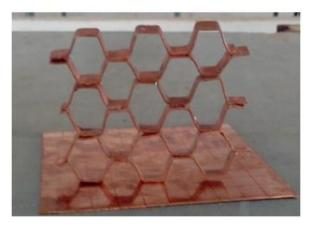
Figure 3. Copper Honeycomb core fabricate.
