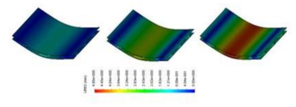
Figure 7. Deflection plots for various loads with core height of 5mm
