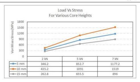
Figure 9. Variation of Von Mises Stress with core height.
