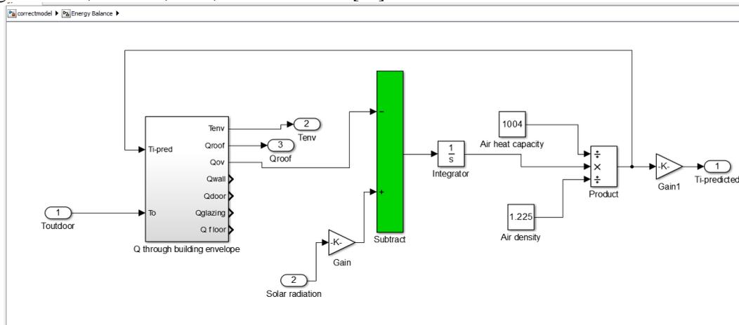
Figure 3. Block diagram of the energy balance in SIMULINK
