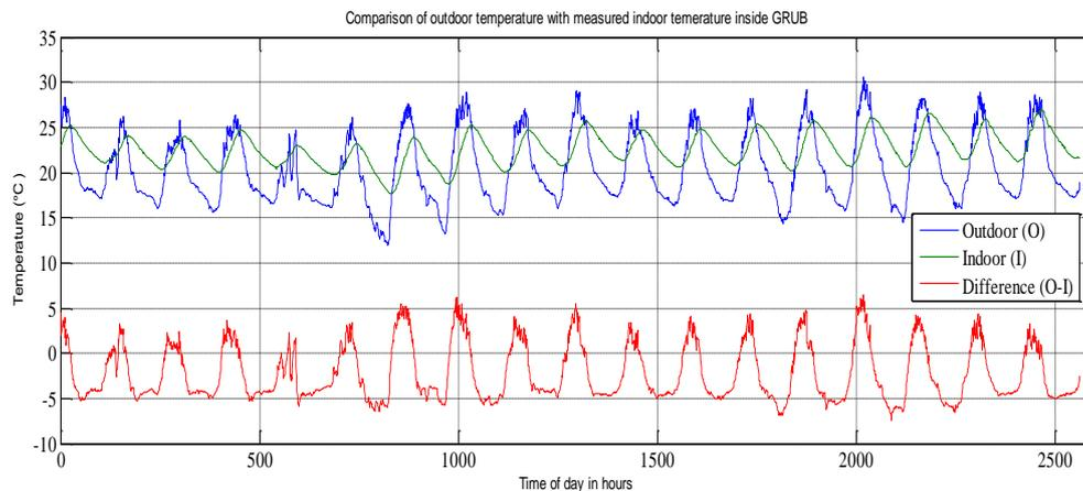
**Figure 5.** Graph showing the measured outdoor temperature and the measured indoor temperature inside the GRUB.
