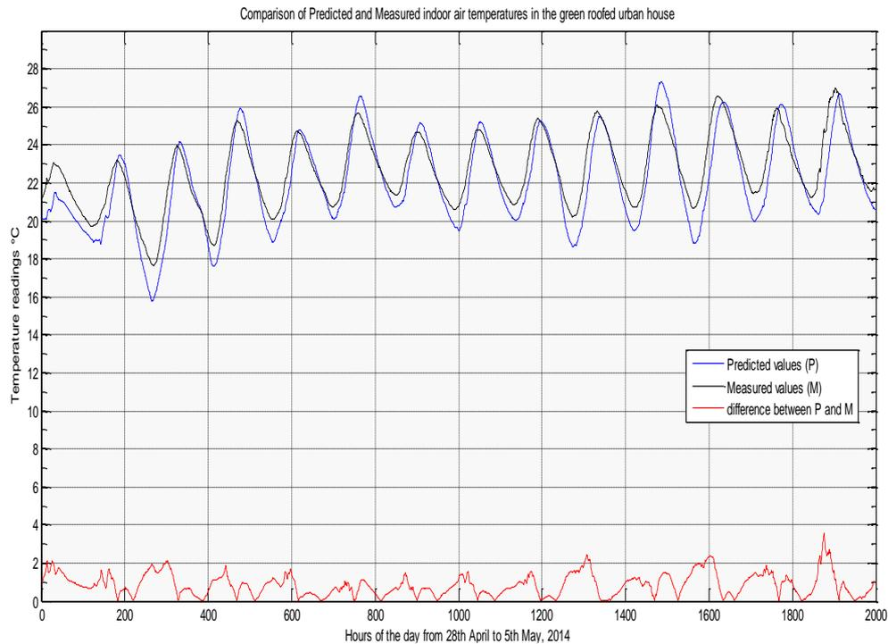
**Figure 4.** Graph showing the predicted air temperature from GRUBCLIM, the measured value and the difference at each point of the two values.
