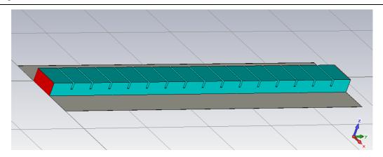
Figure 8: the dielectric-waveguide (DW) with upper notches filter with no. of gating = 16
