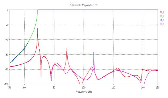
Figure 7: s-parameter of dielectric waveguide WR-2.5
