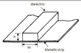
Figure 1: Typical micromachined Dielectric waveguide
