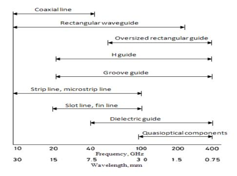
Figure 2: Useful ranges of millimeter waveguide
