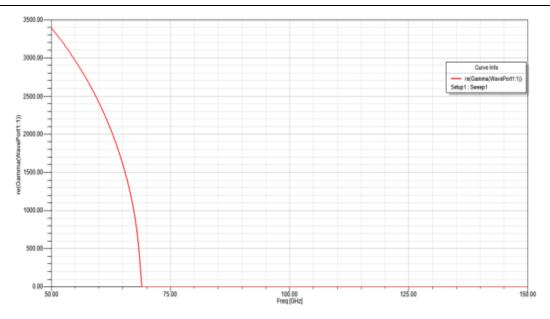
Figure 6: attenuation constant of dielectric waveguide WR-2.5
