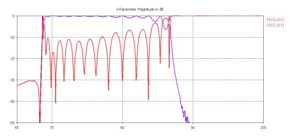
**Figure 9:** Dielectric-waveguide filter response with no. of gating = 16
