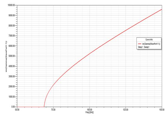
Figure 5: propagation constant of dielectric waveguide WR-2.5
