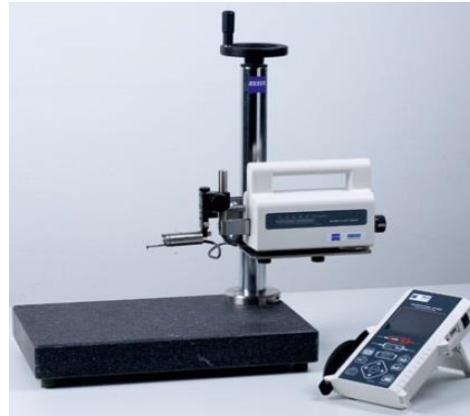
Figure. 6: Surfcom flex surface roughness measuring machine
