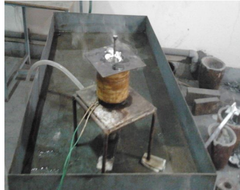
Figure 3: Electric coil vibration
