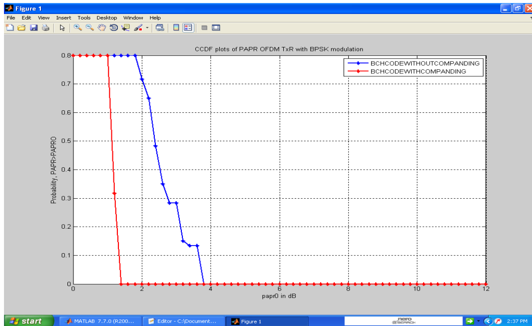
Fig. 4 CCDF plots for BCH codes with and without companding.
