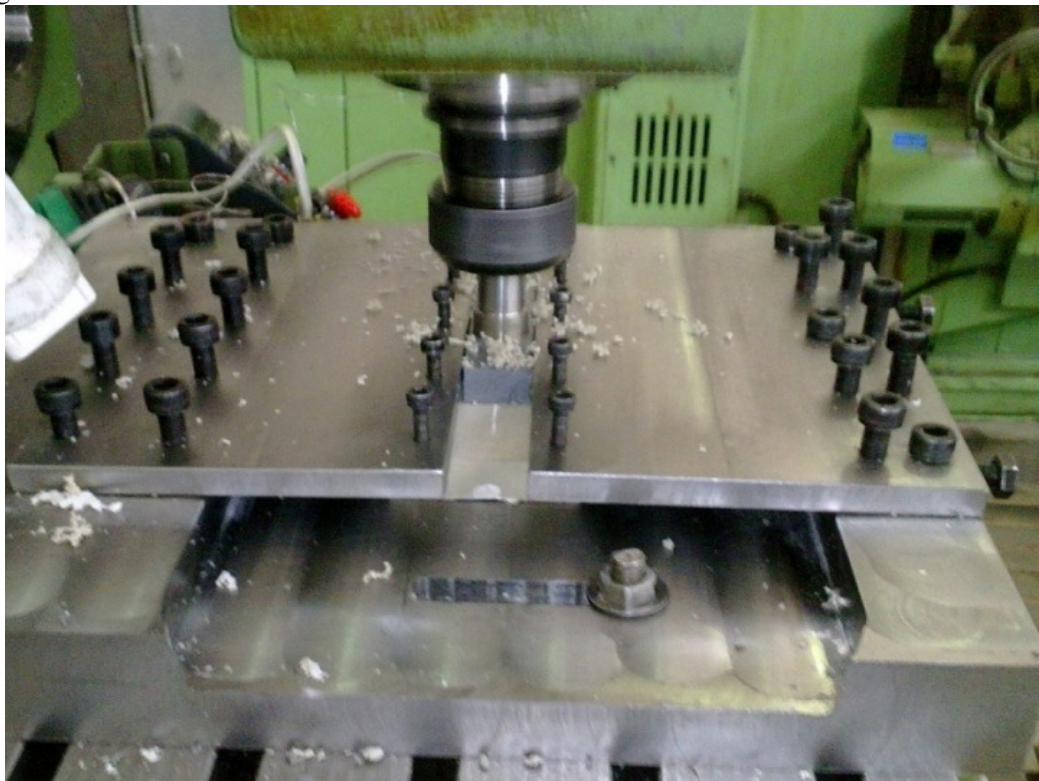
Figure 2. producing of \text{Al}_2\text{O}_3/\text{PP} nanocomposite via novel friction stir processing technique
