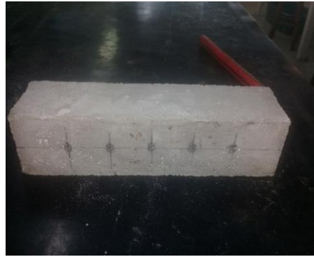
Figure 1. Position of the ultrasonic readings on the specimens.
