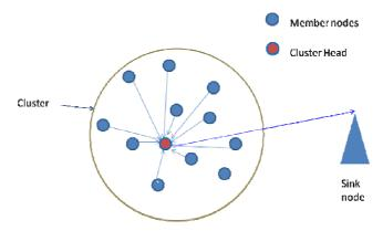
Figure 3. Each cluster have a CH and information receive from member nodes
