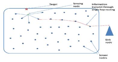
Figure 1. Target tracking using HCTA and single hop routing scenario.
