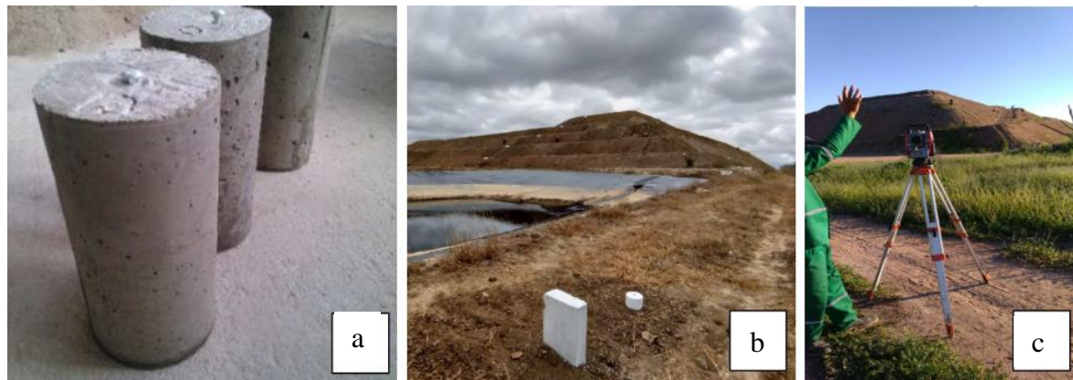
Figure 3 - Instrumentation used to monitor landfill displacements: (a) surface markers; (b) fixed point; (c) total station
