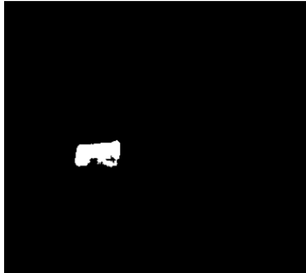
Fig.4 Binarized image showing the yellow marker. Here the original image is binarized with values to make yellow color highlight & background black.
