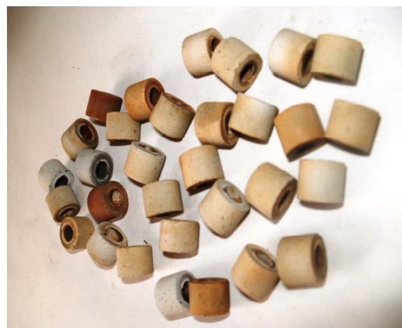
Figure 3: \text{Al}_2\text{O}_3 coated specimens affected by erosive wear
