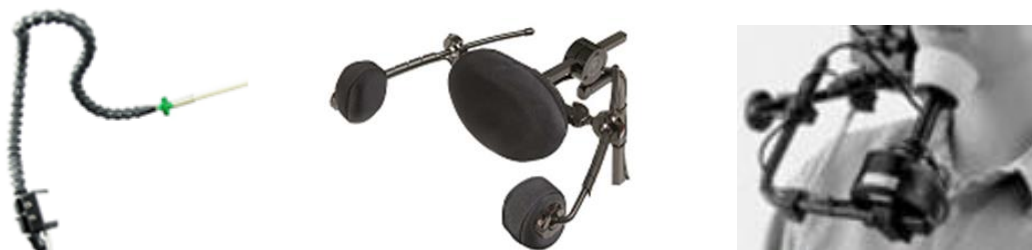
Figure 3. Commercial interfaces: (a) Sip-and-puff (b) headrest (c) chin joystick [15]
