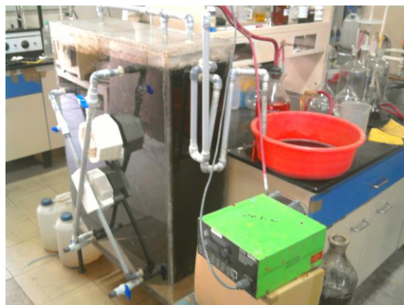
Fig 2. Inclined Tube Reactor for Leachate Treatment (Actual Set up)
