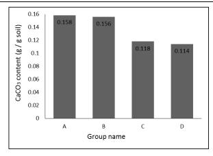
Fig.7 Effect of Calcium source and soil type on the calcium carbonate content
