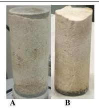
Fig.4 The soil samples after treatment A. Yangtze river sand B. Silica sand
