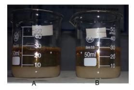
**Fig.5** The calcite precipitation from two different calcium sources A. CaCl<sub>2</sub> (egg shells) and B. CaCl<sub>2</sub> (analytical grade)
