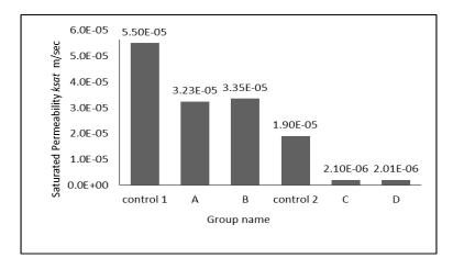
Fig.8 Effect of calcium source and soil type on the permeability
