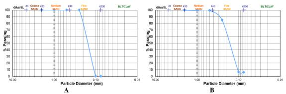
Fig.1 Particle size distribution of the A. Silica sand and B. River sand
