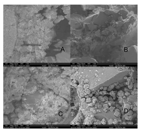
Fig.10 CaCO<sub>3</sub> crystals images (SEM) of treated samples of different calcium sources and soil types
