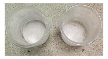
**Fig.6** The calcite precipitation from two different calcium sources after drying A. CaCl<sub>2</sub> (egg shells) and B. CaCl<sub>2</sub> (analytical grade)
