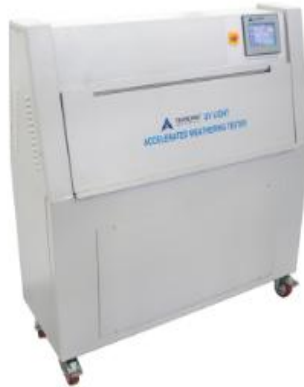
FIG 4: Weathering Test apparatus (image © Presto Group)
