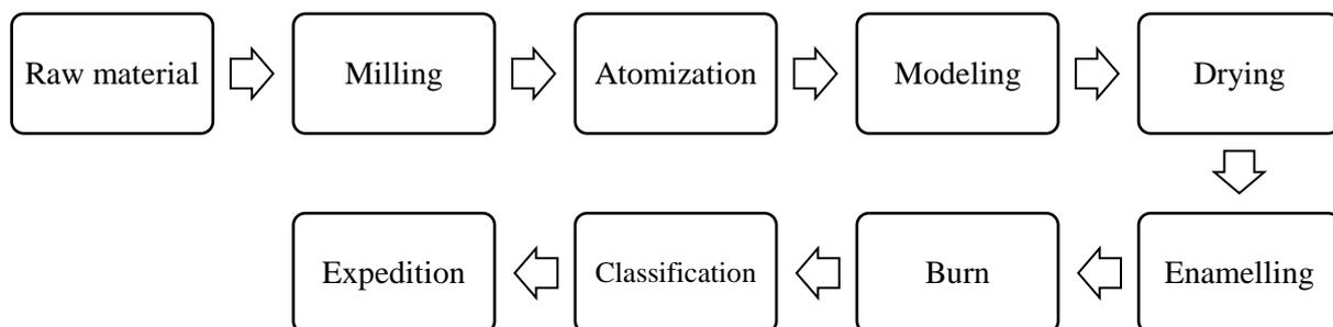
**Figure 01:** flow chart of the manufacturing process of ceramic tiles
