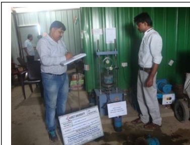
Activity : CBR Testing of JJR1 at Ch- 950 LHS
