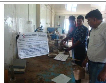
Activity :Atterberg Limits of JJR1 at Ch-750 LHS
