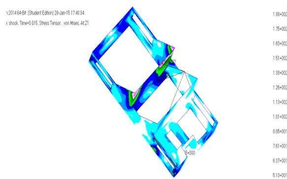
Figure 3 - Shock von mises stress on z direction =113 Mpa
