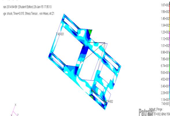
Figure 1 - Shock von mises stress on x direction =110 Mpa
