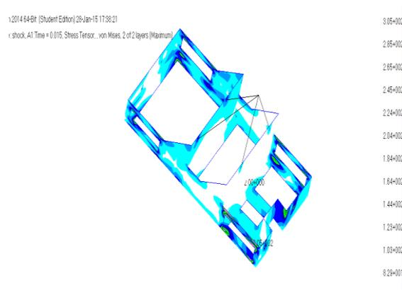
Figure 2 - Shock von mises stress on y direction =184 Mpa
