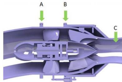
**Figure 4.** Position of anticavitation valves
