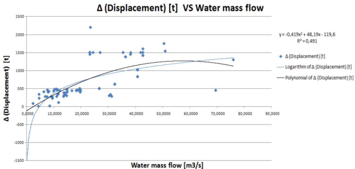
Figure 9. Vessel displacement vs. water mass flow
