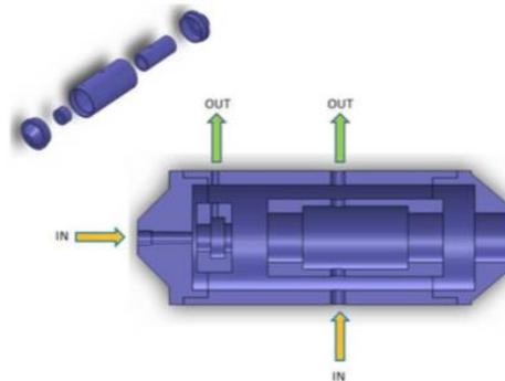
**Figure 5.** Rotary joint with inlets and outlets of oil
