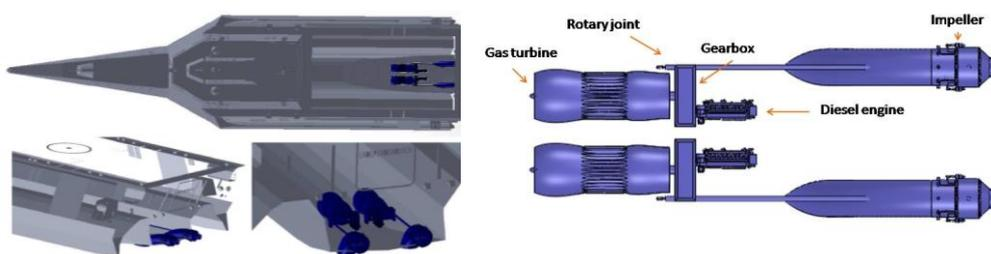
Figure 11. Adaptation of HyLife in the LCS (left) and propulsion plant lay-out (right)
