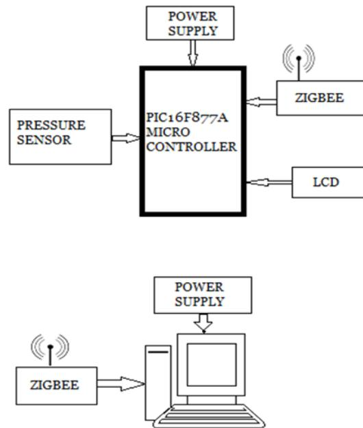
Figure 1: Functional Block of the System
