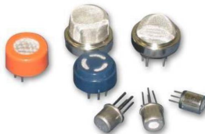
Fig. 8. Metal-oxide semiconductors (MOS) sensors
