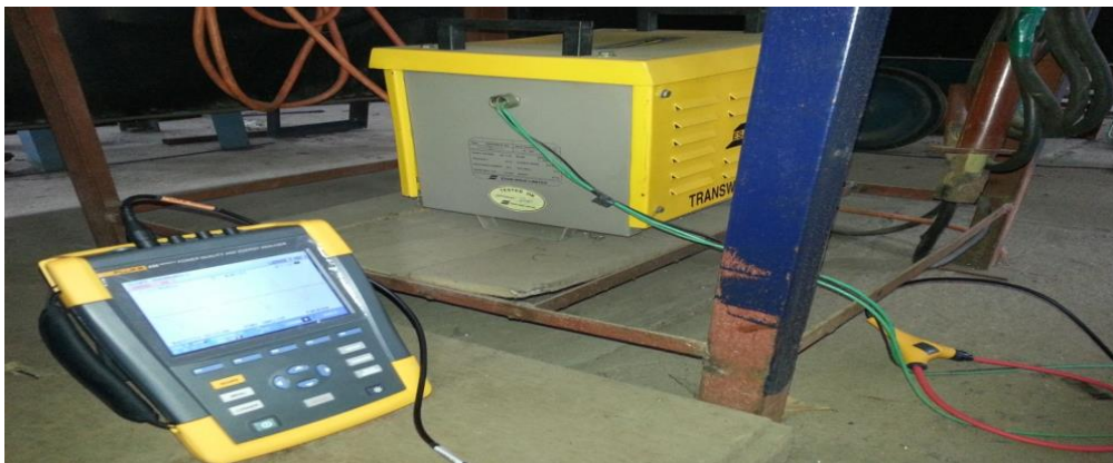
Figure 24: Experimental setup to capture welding current waveforms
