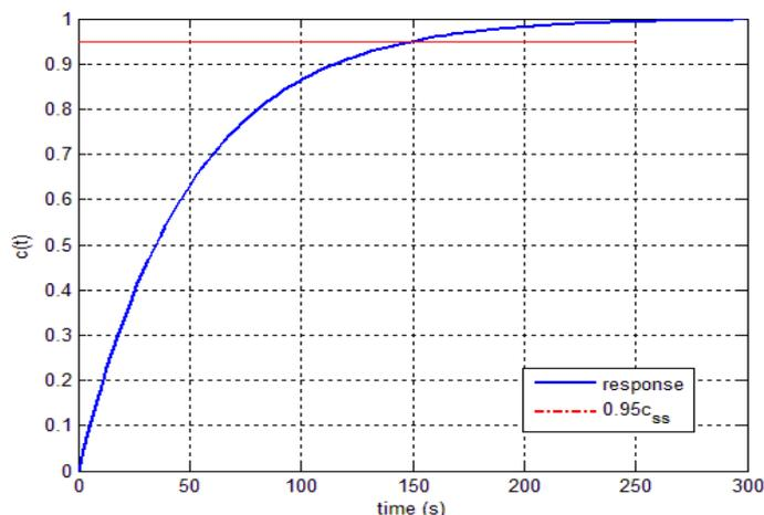
Figure1. Step response of the uncompensated process.
