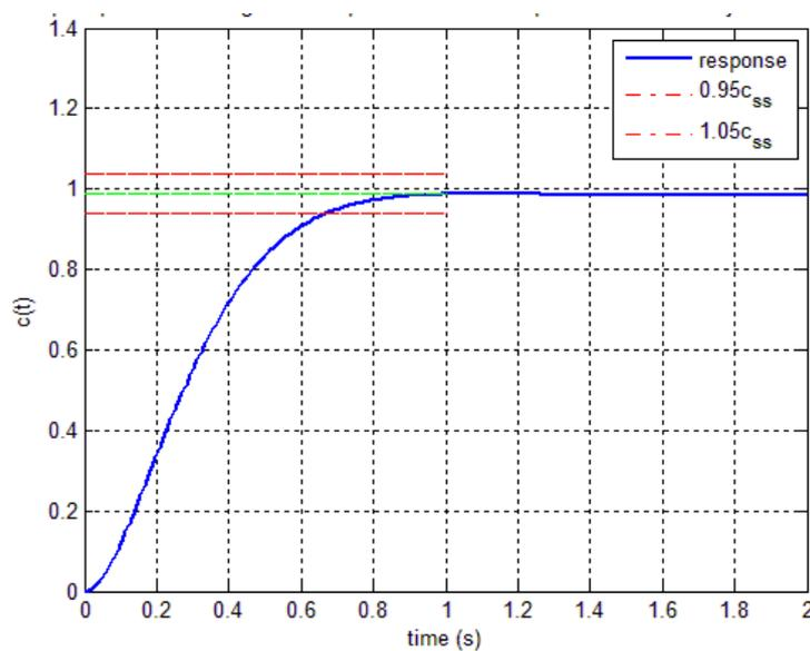
Figure 2. Step response of the lag-lead compensated system.
