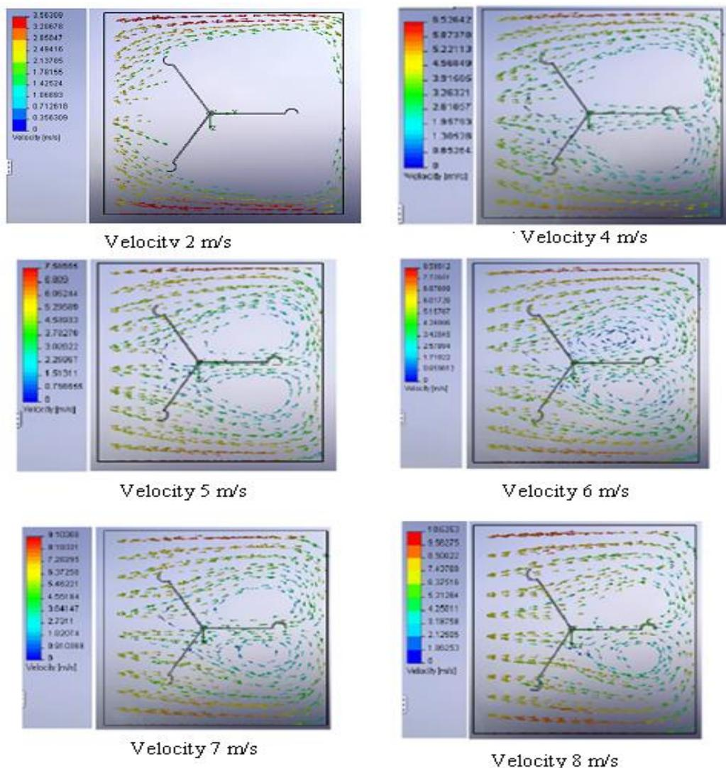
Figure 4. Flow pattern for velocity V= 2 m/s to 8 m/s
