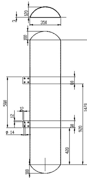
Figure 3. Modified shape of Savonius rotor of Savonius turbine
