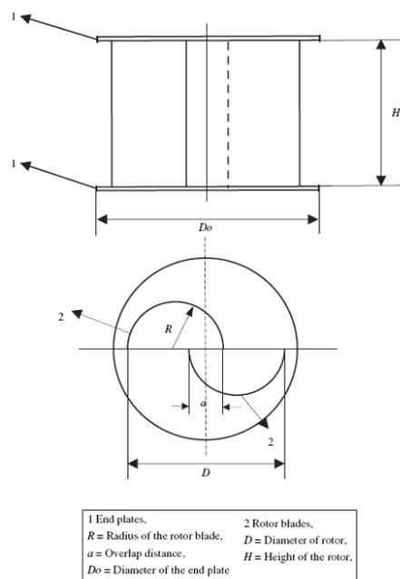
**Figure 1:** Basic Structure of a Conventional Savonius Rotor[1]
