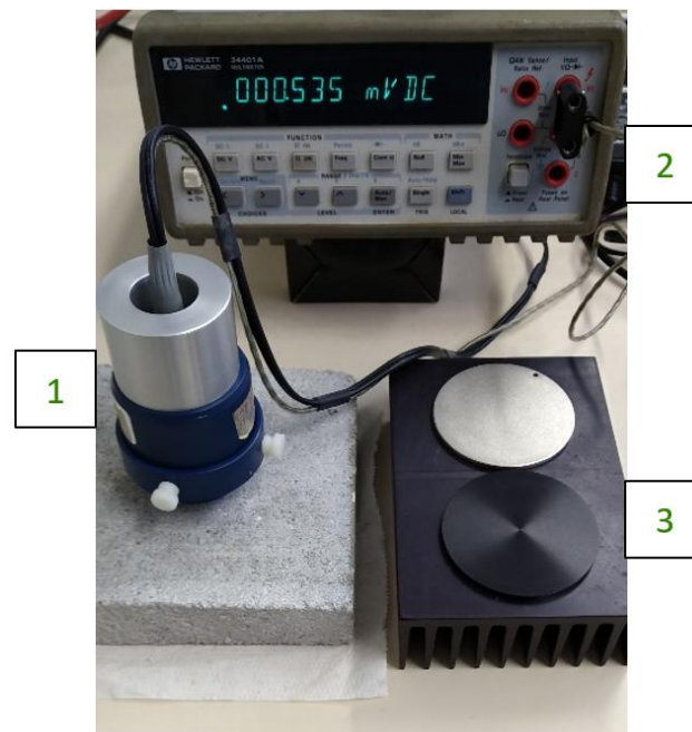
Figure 3: Portable emissometer components: 1) Detector; 2) Multimeter; 3) Calibration Standards
