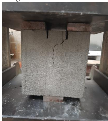
Figure 4: Failure exiting the notch.
