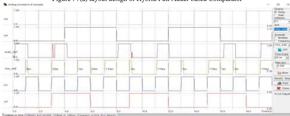
Figure : 7(b) simulation result of Hybrid Full Adder based Comparator
