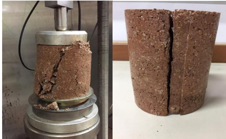
Figure 12: Rupture of specimens: (a) UCS test; (b) Tensile Strength test.
