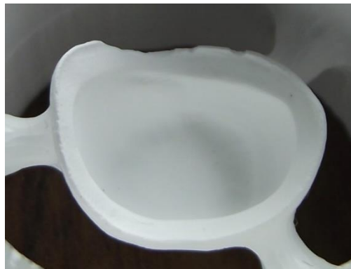
Figure 4. Damages caused to the border of the workpiece during finishing
