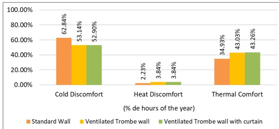
**Figure 9.** Thermal comfort, cold discomfort and heat discomfort for the three simulated models
