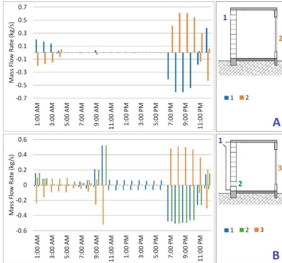
**Figure 15.** Mass flow rate during the Summer Solstice for the model with the common wall (A) and for the model with the Trombe wall (B). Negative values mean that the air is leaving the internal zone
