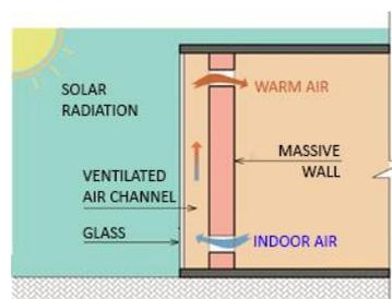
**Figure 1.** Ventiladed Trombe wall. Adapted from Abbassi et al. [3]
