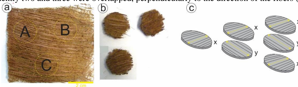
Figure 2. Samples used in the acoustic absorption test: (a) a sample used for the acoustic absorption test; (b) the three circumferences A, B and C taken from the sample; (c) scheme showing the way the circumferences were overlapped and the direction of the fiber arrangement (x, y).
