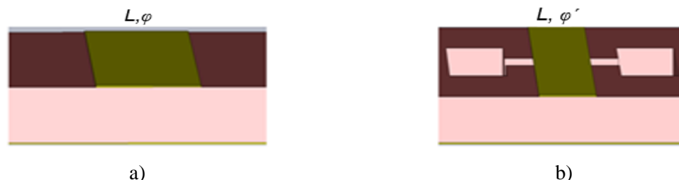
Figure 1: The model of normal microstrip line (a) and microstrip line with DSS
