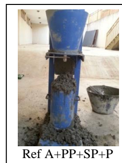
Fig 8 : Compacting factor of ACI mix design and Dreux Grossier formulation.
