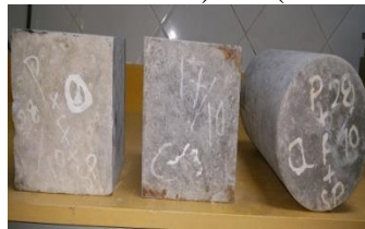
Fig 2: Control Sample and Penetron Admix Samples.
