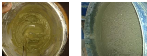
Fig 1: Penetron Admix mix (left) and Ref E+PP+SP+P (right).
