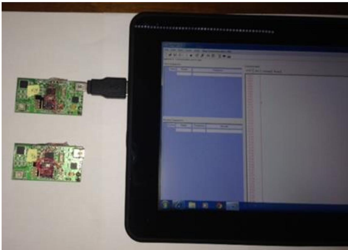
**Figure 5.** The transmitter and the receiver sensors with the coach's tablet.
