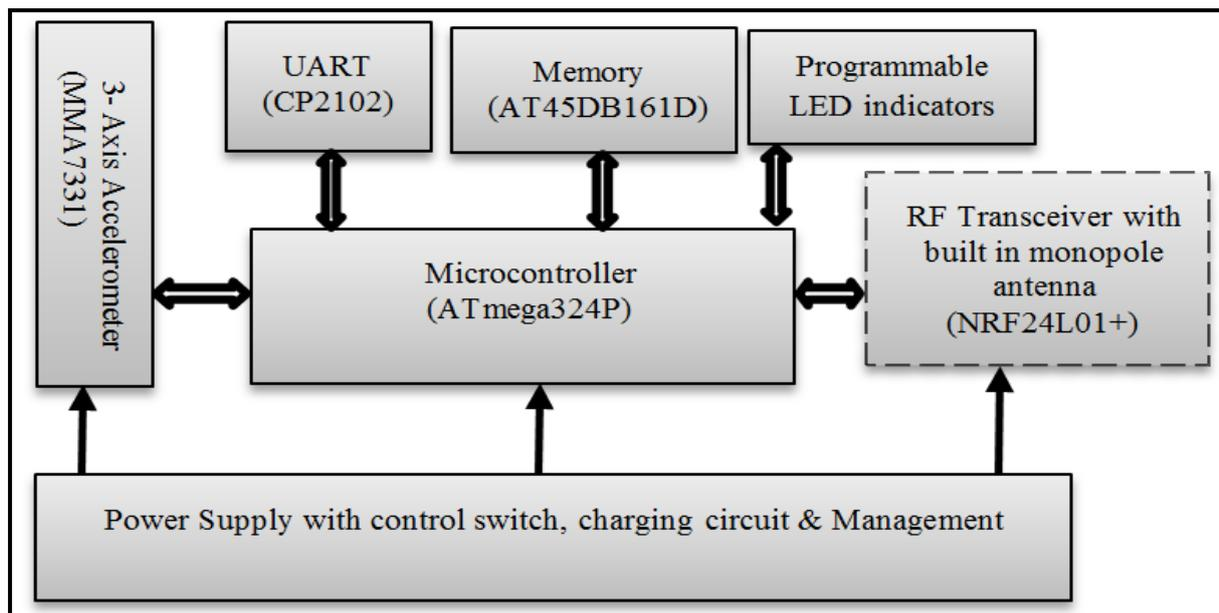
**Figure 1.** Block diagram of the nCore 2.0 & 3.0. The dotted line block represents the module that is added to the wearable wireless sensor nCore 2.0 [3-7].
