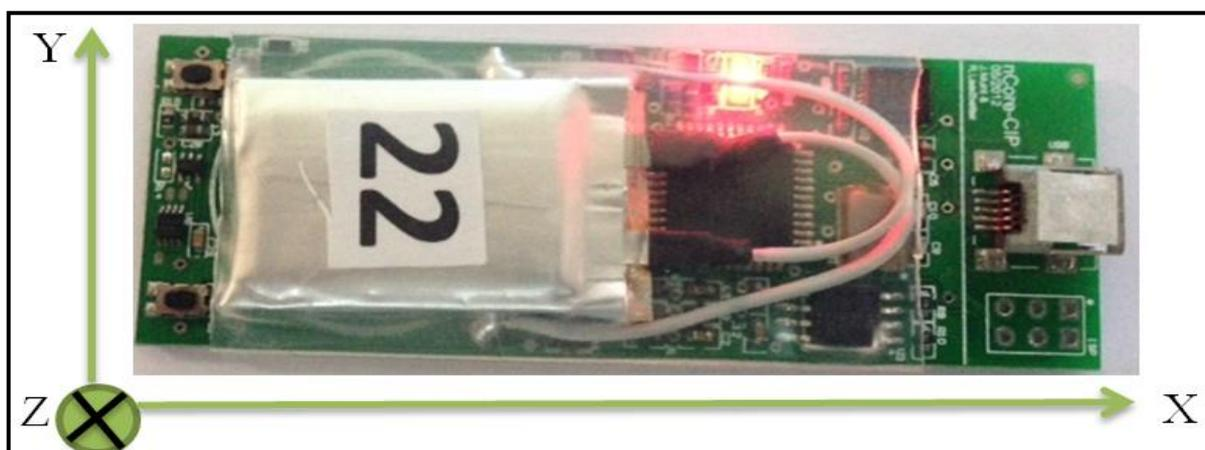
**Figure 2.** nCore 3.0 wearable wireless sensor.
