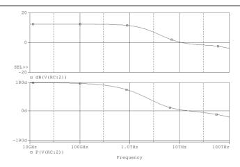
Figure 12. Bode diagrams of CS CNTFET amplifier with SPICE.
