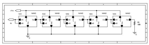
Figure 14. Schematic of the circuit used to simulate the behaviour of the NAND gate.
