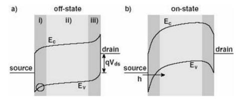
Figure 5. Band diagrams for a SB-CNTFETs in the 'off' and 'on' states respectively.
