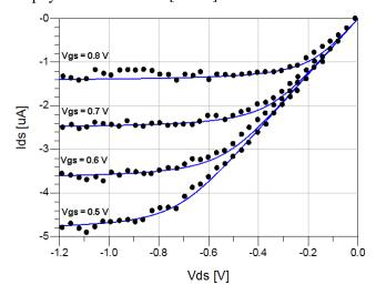
**Figure 9.** Simulated  $I_{ds} - V_{ds}$  characteristics (denoted by continuous lines) and experimental ones [22] (denoted by  $\bullet$ ) (from [2]).
