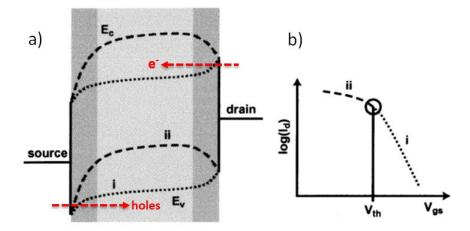
Figure 6. a) Subthreshold band diagrams for SB-transistors; b) I-V characteristics in subthreshold condition.
