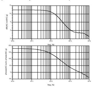
Figure 13. Bode diagrams of CS CNTFET amplifier with Verilog-A .
