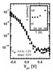
**Figure 7.** Experimental I<sub>d</sub> versus V<sub>gs</sub> subthreshold characteristics for a p-type transistor, with a channel length of 300 nm and a gate oxide thickness of 20 nm (*from* [18]).
