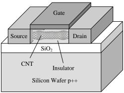
**Figure 8.** 3D representation of a C-CNTFET.
