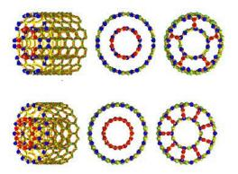
**Figure 2.** Structure of a MWCNT.
