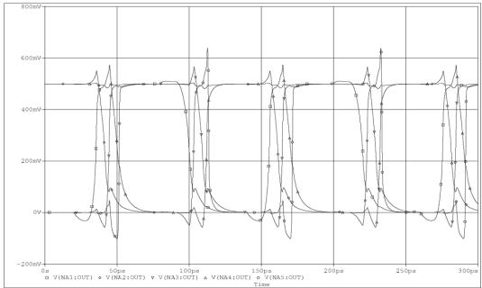
**Figure 15.** Transfer function of the circuit shown in Fig. 16 with SPICE, measured at the gate of first, second, third and fourth NAND, marked with circles, crosses, squares and triangles respectively.
