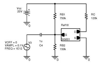
Figure 11. A CNTFET amplifier in CS configuration.
