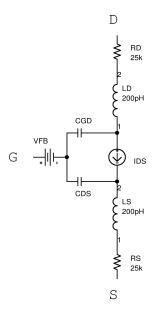
Figure 10. Equivalent circuit of a n-type C-CNTFET (from [3]).
