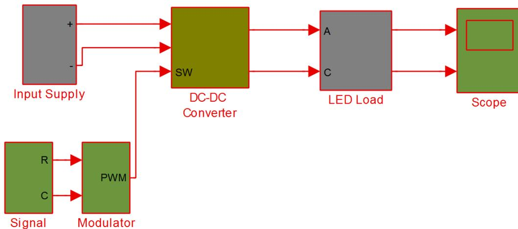
**Figure 5.** MATLAB-SIMULINK model of Buck-Boost/SEPIC Converter
