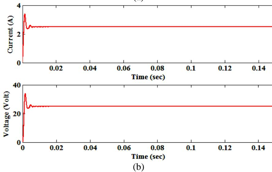
Figure 7. Dynamic response of current and voltage in SEPIC Converter at 30% and 70% duty cycle for  $V_g$  at 12V and  $R$  at 10 $\Omega$ .
