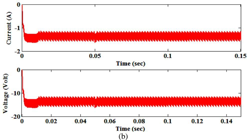
**Figure 9.** Dynamic response of current and voltage in Buck-Boost Converter at 30% and 70% duty cycle for  $V_g$  at 12V and R at  $10\Omega$ .
