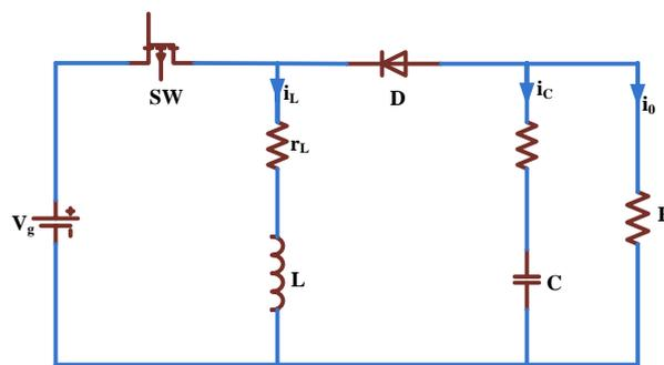
Figure 3. DC-DC buck-boost converter
