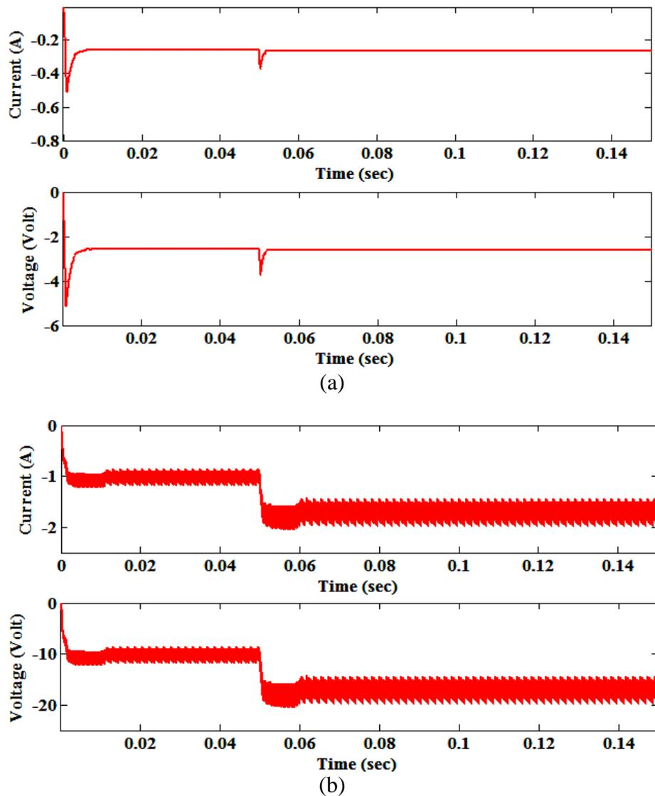
**Figure 8.** Dynamic response of current and voltage in Buck-Boost Converter at 30% and 70% duty cycle for  $V_g$  varies from 9V to 15V and R at 10Ω.
