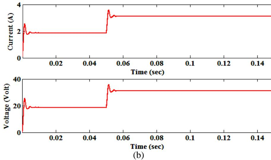
Figure 6. Dynamic response of current and voltage in SEPIC Converter at 30% and 70% duty cycle for  $V_g$  varies from 9V to 15V and  $R_{at}$  10 $\Omega$ .
