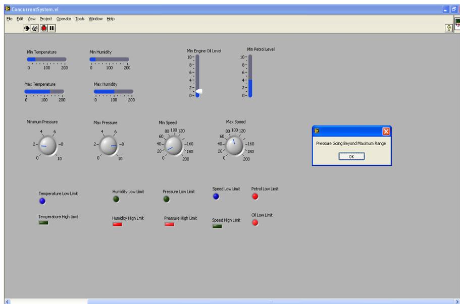
Figure 5. Abnormal Output: Pressure going above maximum
