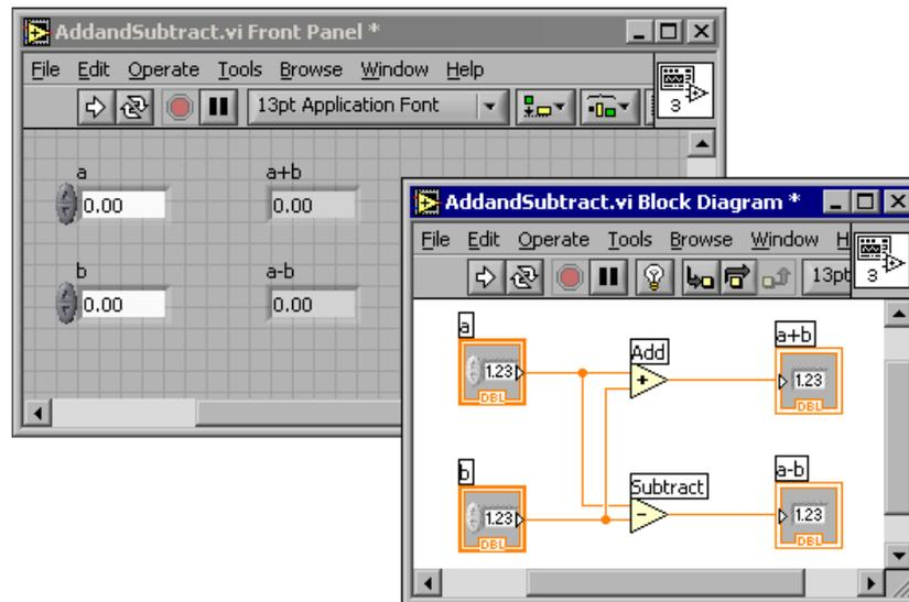
**Figure 1** Example of a block diagram and corresponding Front Panel in LabVIEW
