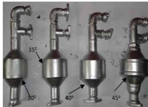
Fig.2 Photographic view of catalytic converters (30°, 35°, 40° and 45°)
