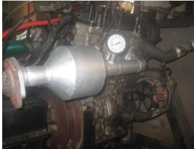
Fig.4 Photographic view of Catalytic converter (40° Cone angle) fitted in the exhaust manifold.
