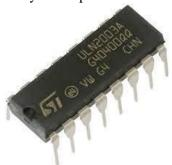
Figure7: ULN2003 IC used in our project
