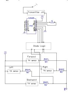
Figure 5: Circuit Diagram of Transmitter Section
