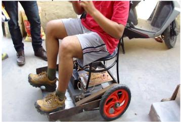
Figure 9: Head Motion controlled wheelchair
