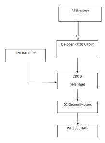
Figure 4: Block Diagram of Receiver section of Head Motion Controlled Wheelchair
