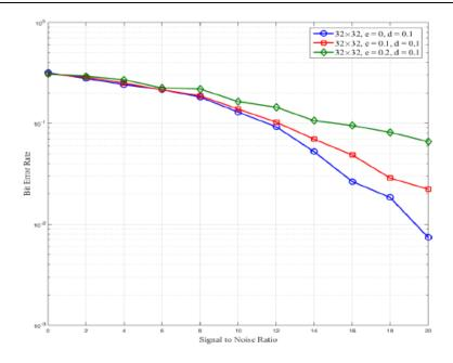
Fig. 4. Bit error rate performance of  $32 \times 32$  multiple-input multiple-output system versus signal to noise ratio (dB) for e=0,0.1,0.2 and d=0.1
