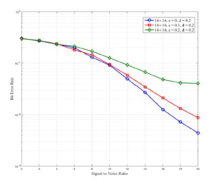
Fig. 2. Bit error rate performance of  $16 \times 16$  multiple-input multiple-output system versus signal to noise ratio (dB) for e = 0, 0.1, 0.2 and d = 0.2
