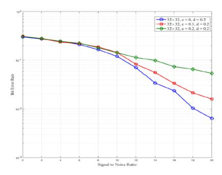
Fig. 5. Bit error rate performance of  $32 \times 32$  multiple-input multiple-output system versus signal to noise ratio (dB) for e=0,0.1,0.2 and d=0.2
