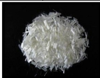
Fig. 1 Physical appearance of short Polyester fibres
