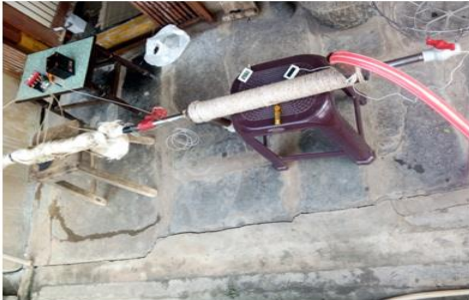
Fig.5. Experimental setup of heat exchanger with corrugated twisted pipe
