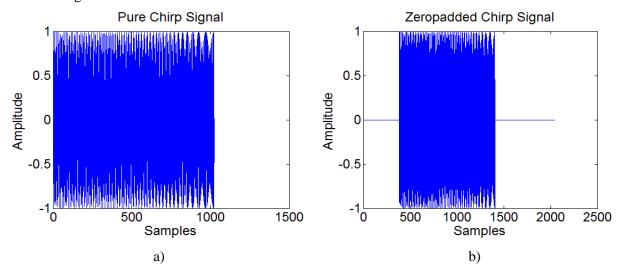
Figure 1. a) Pure Chirp Signal and b) Zero-padded Chirp Signal
