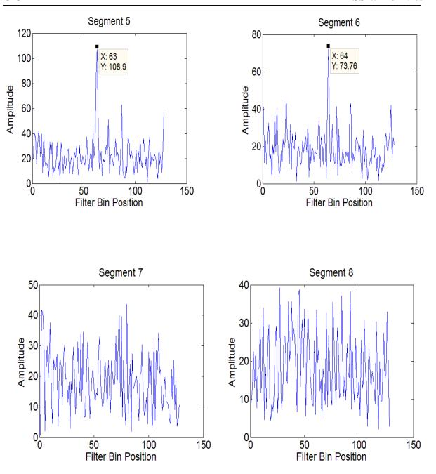
Figure 4: Representation of the Output of Eight Segments of Noisy Chirp Signal
