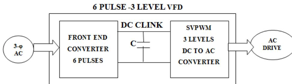
Figure 12: 6 Pulse-3 levels SVPWM VFD
