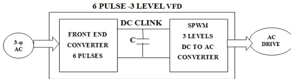
**Figure 3:** 6 Pulse-3 levels SPWM VFD
