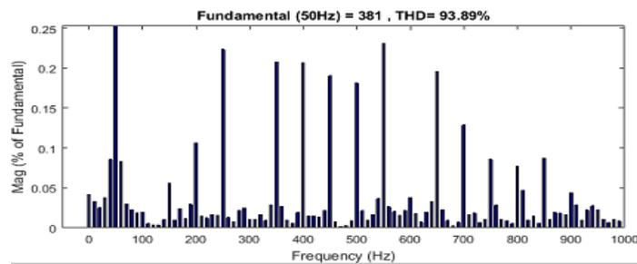
Figure 36 : Inverter output Voltage FFT
