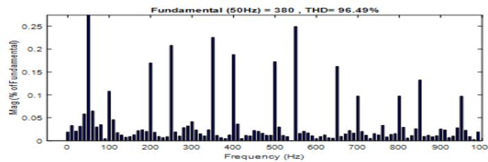
Figure 18 : Inverter output Voltage FFT
