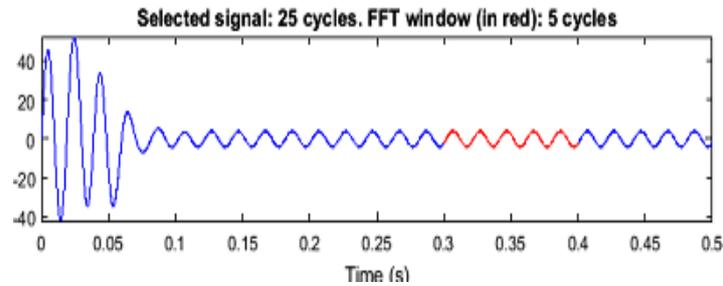
Figure 37: Motor Supply Current
