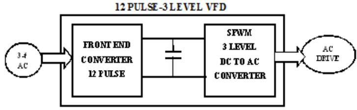
Figure 21:12 Pulse-3 levels SPWM VFD
