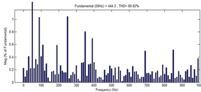
Figure 9: Inverter output Voltage FFT
