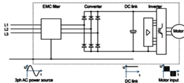
Figure 1: Topology of a 3ph PDS
