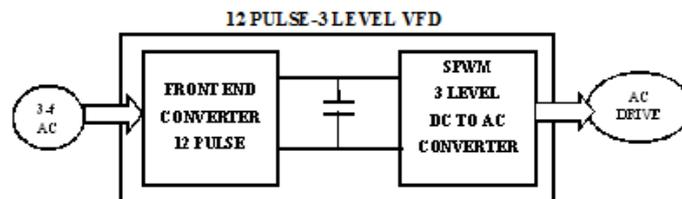
Figure 30 :12 Pulse-3 levels SVPWM VFD
