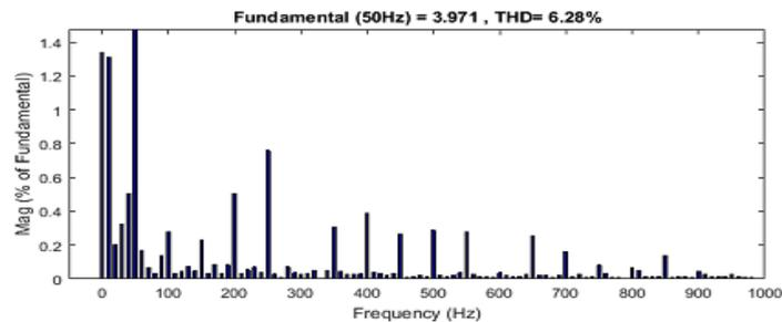
Figure 38: Motor Supply Current FFT
