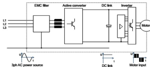
Figure 2: 3ph PDS with active front converter
