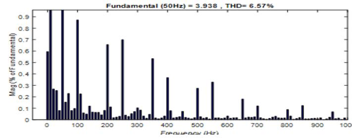
Figure 20: Motor Supply Current FFT
