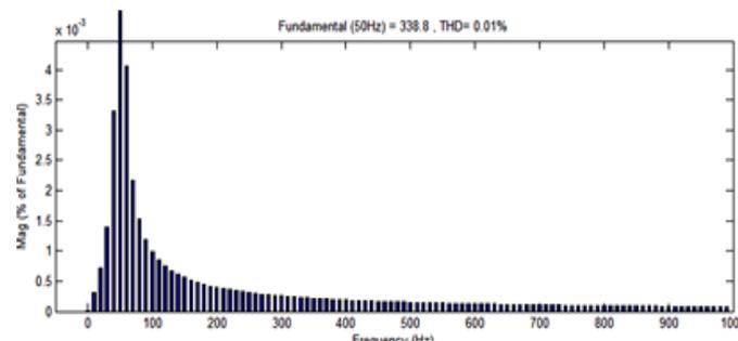
**Figure 7 :** Supply Voltage FFT
