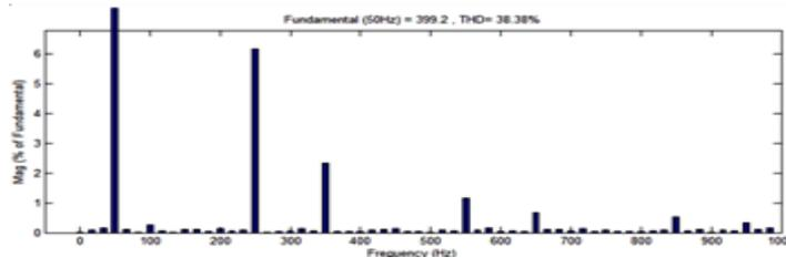
Figure 27 : Inverter output Voltage FFT
