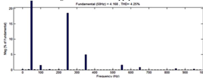
Figure 29: Motor Supply Current FFT
