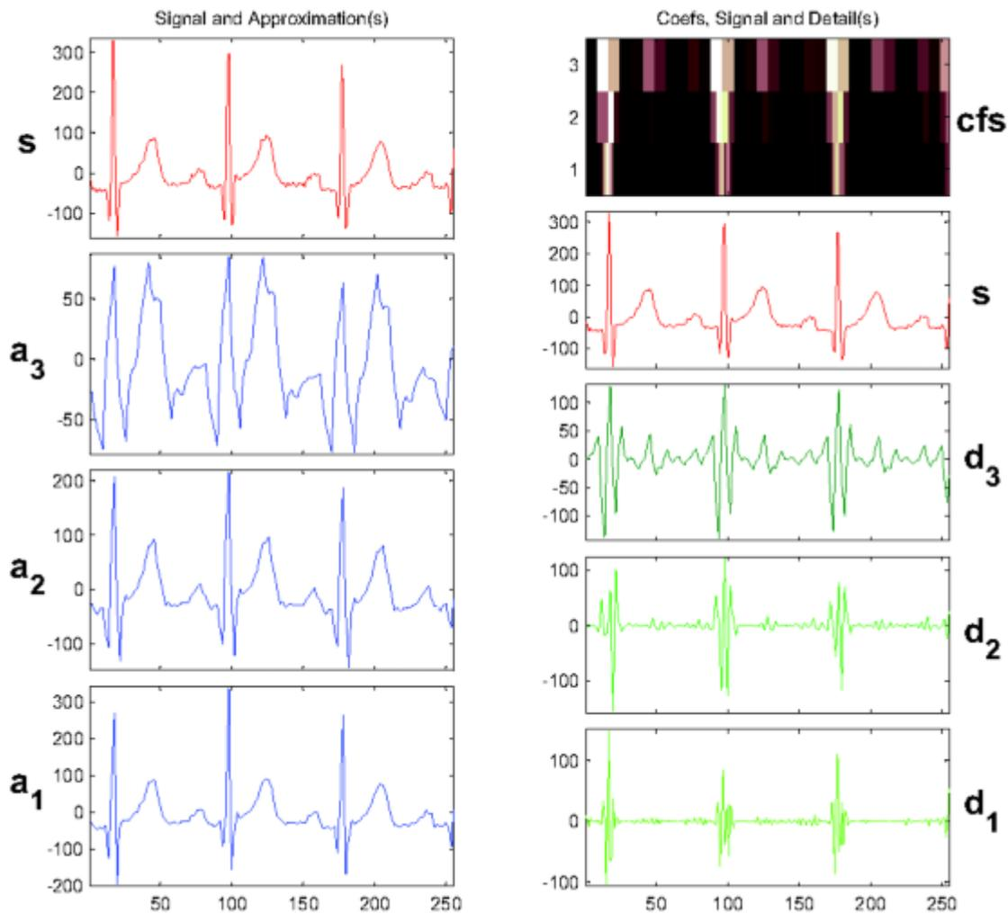
Figure 4: wavelet decomposition using Daubechies wavelet of order 3
