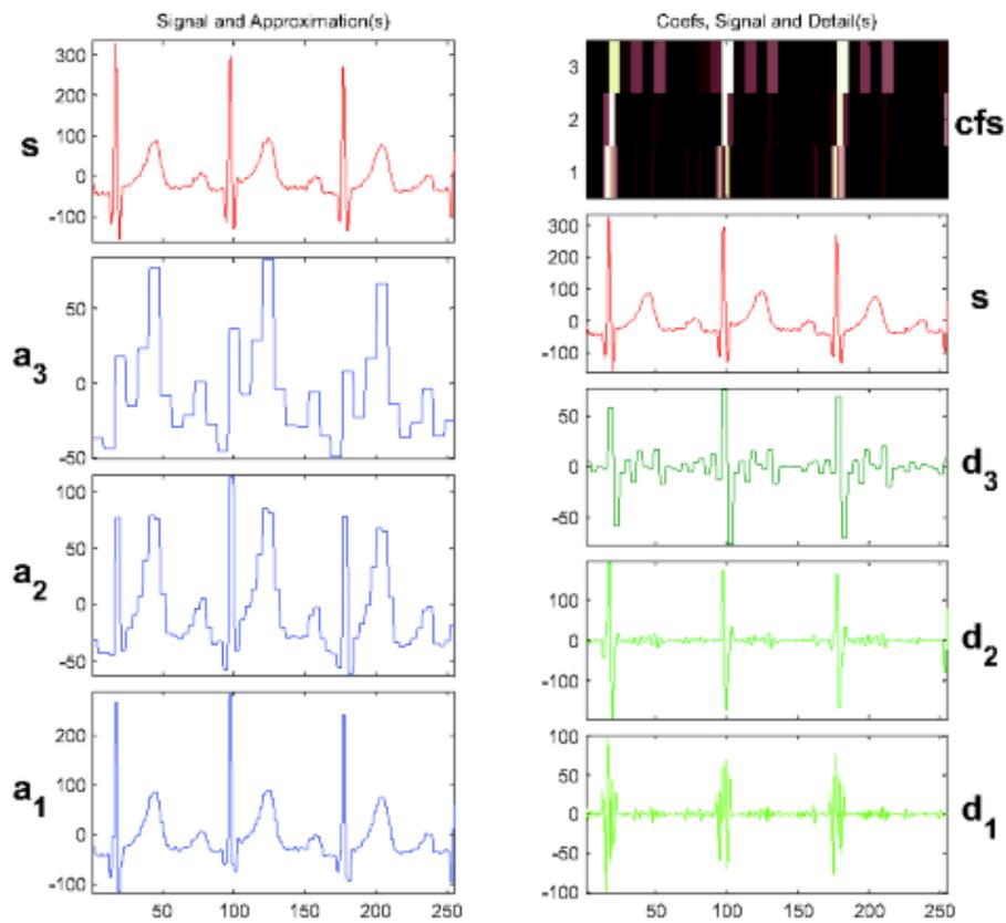
Figure 3 : wavelet decomposition using Daubechies wavelet of order 1
