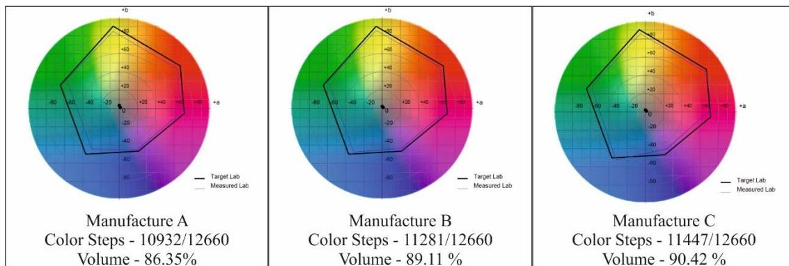
Or concluding results from test results we select Cyan ink of Manufacturer A, Yellow ink from Manufacturer B and Magenta and Black Ink from Manufacturer C. Final test print using selected combination are printed and again examined using X rite instruments. The test shows final Conclusion for find optimised ink set to produce maximum color volume of gamut for color reproduction.
