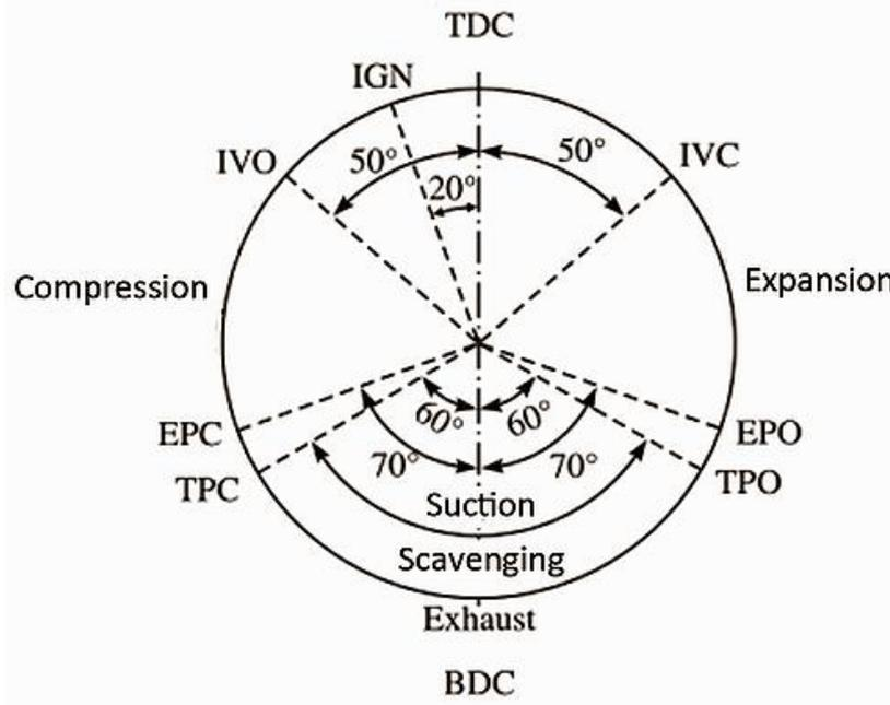
Figure 3: Port Timing Diagram of Two Stroke Engines
