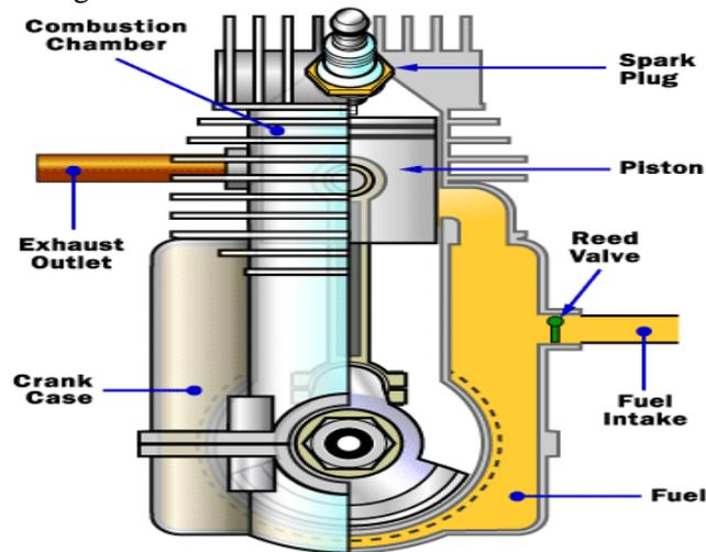
Figure 1: Two Stroke Engine Components
